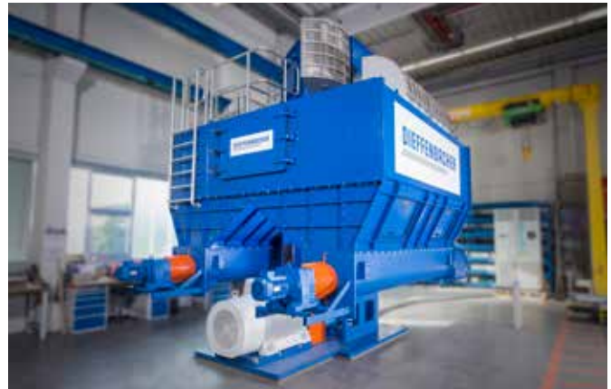
Flameless explosion venting on a grinder machine.
