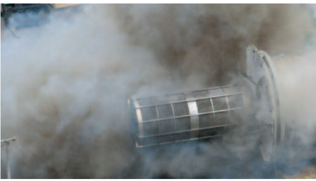
Aluminum dust explosion with an indoor venting system installed
