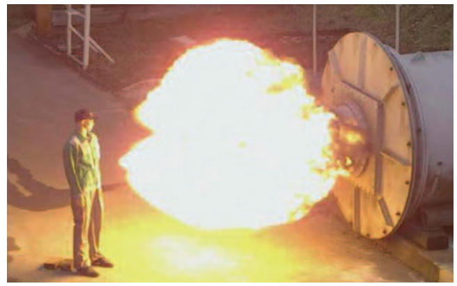
Flame length of an aluminum dust explosion without an indoor venting system installed
